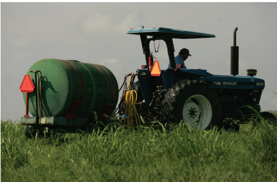
Maintenance crews at Acadiana Airport use a tank sprayer attached to a tractor to spray bahiagrass, smutgrass and other problem weeds. Their spray program has reduced the time and money required for mowing each year.
