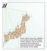
**Geodetic surveys** take into account the shape and size of the earth when distances are long and must curve to accurately describe the land.
