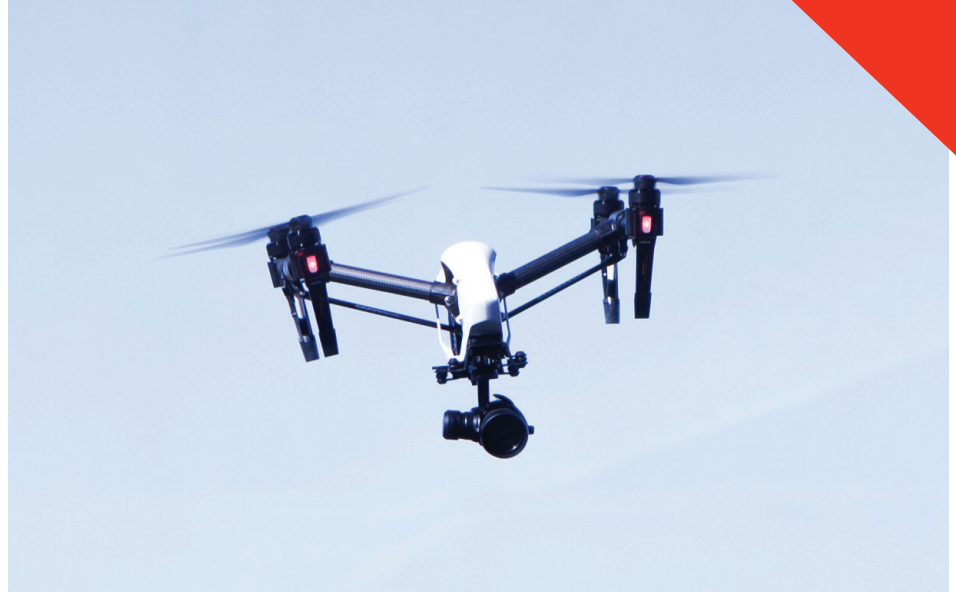
Well-suited to small collection areas and those that need to be regularly flown, UAS makes it possible to collect detailed spatial data over locations that are dangerous or inaccessible.
