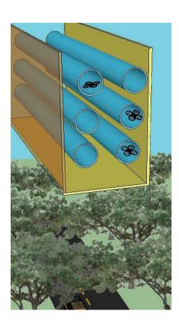
This illustrates an avigation easement dedicated to automated unmanned aircraft. This easement contains six individual flight lanes (shown in blue).
