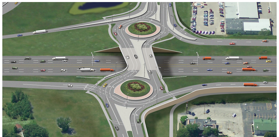
Since roundabouts are proven to dramatically reduce traffic incidents, they are one of the many enhanced safety features that are a part of the US 41 Project.
