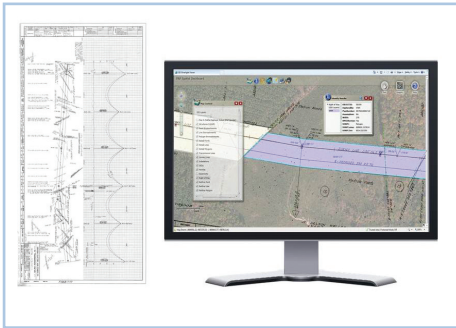
From start to finish: Plans and profiles are scanned, georeferenced and then digitized into GIS.
