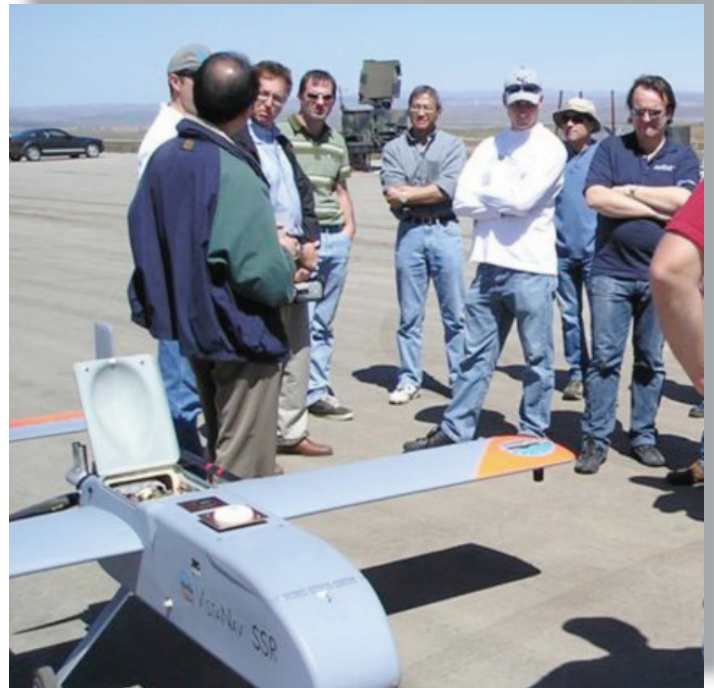
The drone's 2.6 meter wingspan makes it easily transportable from one location to the next.
