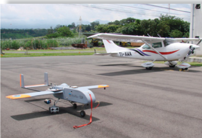
Remotely piloted aerial patrol drones can provide recorded video monitoring and is equipped with anomaly detection software to provide real time detection of high risk targets within the corridor. Photos courtesy of Vector P USA.
