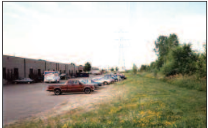
Multiple use of excess land within a 100 foot wide railroad right of way with non-exclusive easements for a pipeline directly under a power line and encroachments for parking within both easements. Also suffers encroachment for snow storage in winter. Available space can accommodate other users within the same easement areas.
