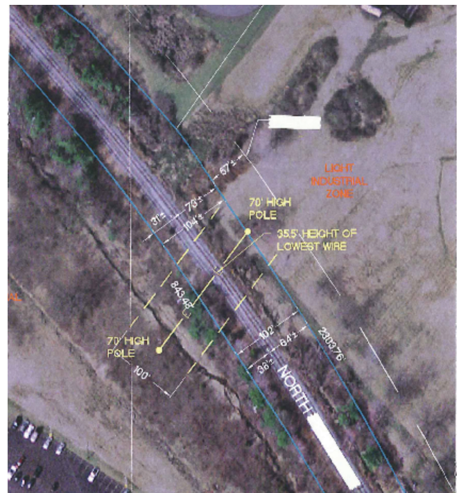
Multiple overhead crossings in an industrial area. Crossings are above specified minimums.
