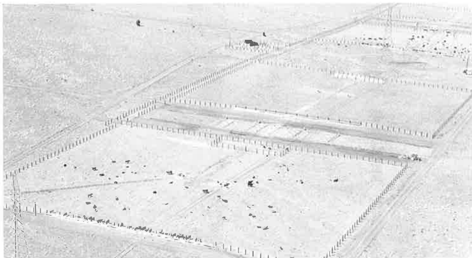
One hundred beef cows and their calves (in two groups of 50) are rotated through four pens beneath the \pm 500 -kV d-c line. Instruments to monitor d-c electric fields and air ions can be seen between the first two pens. Crops are also grown in strips near the instruments. Groups of cattle and crops are also raised under similar conditions in a control area 2,000 feet from the line.
