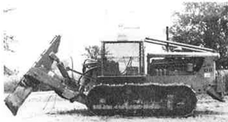
Figure 2. A tractor mounted plow used for burying gas pipelines.
