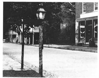
Harpers Ferry shale was used for sidewalk material. Due to the lack of enough shale, brick was used to fill in areas where Harpers Ferry shale should have been. Signs of modern utilities such as man-holes and overhead electrical wires were hidden beneath the street.
