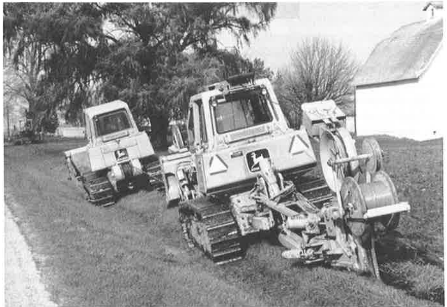
Above: Two John Deere hydrostatic crawlers team up on a fiber optic installation in Illinois. Below: Illinois Bell's John Deere 850 is equipped with hydraulically controlled reel carrier, cable-tension monitoring system and capstan drive.
