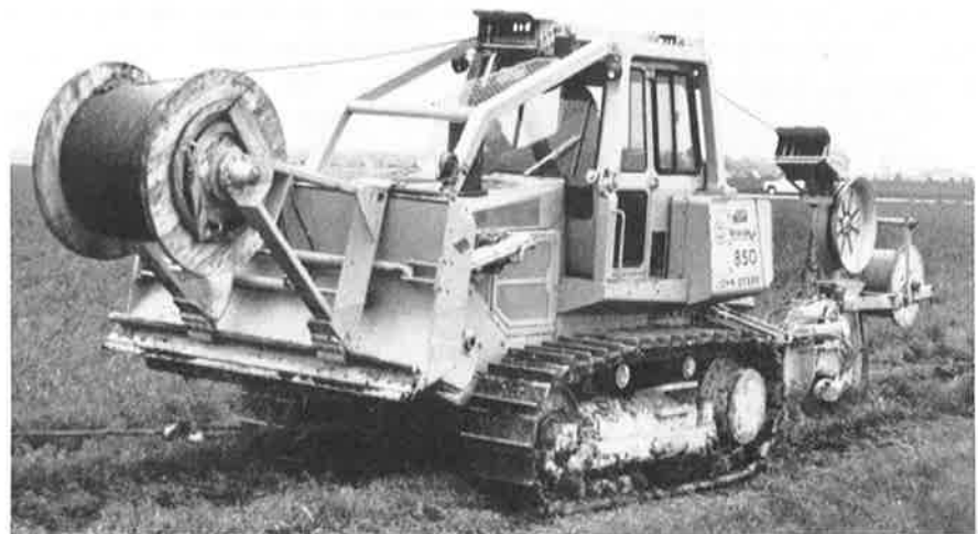
Above: Two John Deere hydrostatic crawlers team up on a fiber optic installation in Illinois. Below: Illinois Bell's John Deere 850 is equipped with hydraulically controlled reel carrier, cable-tension monitoring system and capstan drive.
