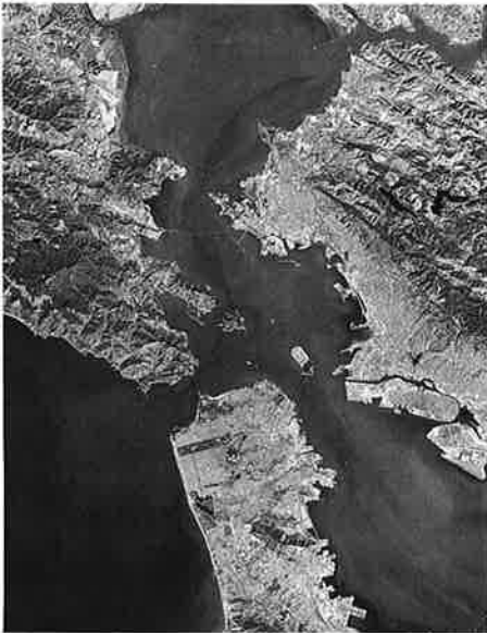
This 500-mile high satellite view of San Francisco was used to generate a land use map for cellular system planning. ©1993 CNES, provided by SPOT Image Corporation.
